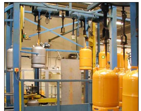
Automatic transfer of cylinders from chain conveyor system to overhead conveyor system
