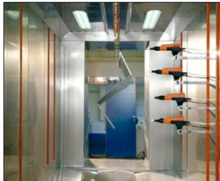
Spray booth for automatic application and recovery of powder paint
