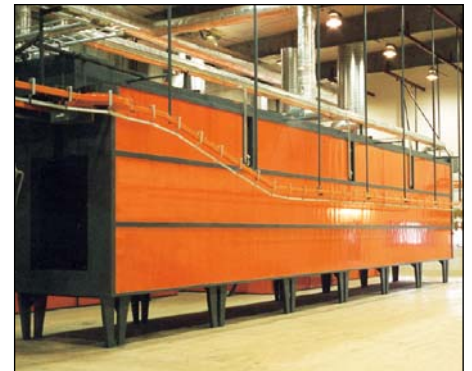
Tunnel oven for drying after pre-treatment, curing/drying wet paint or curing powder paint
