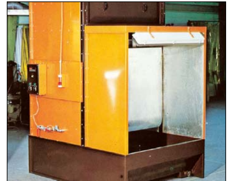
Spray booth for manual application of wet paint
