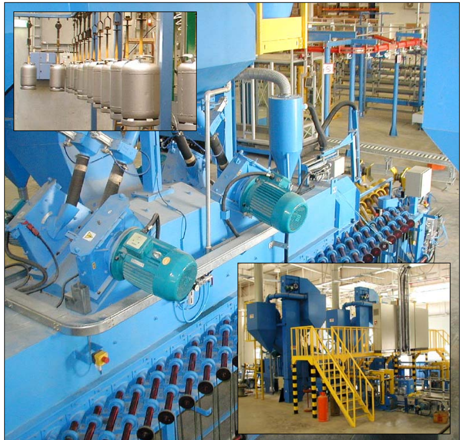
Shotblasting equipment with automatic loading and unloading of cylinders
