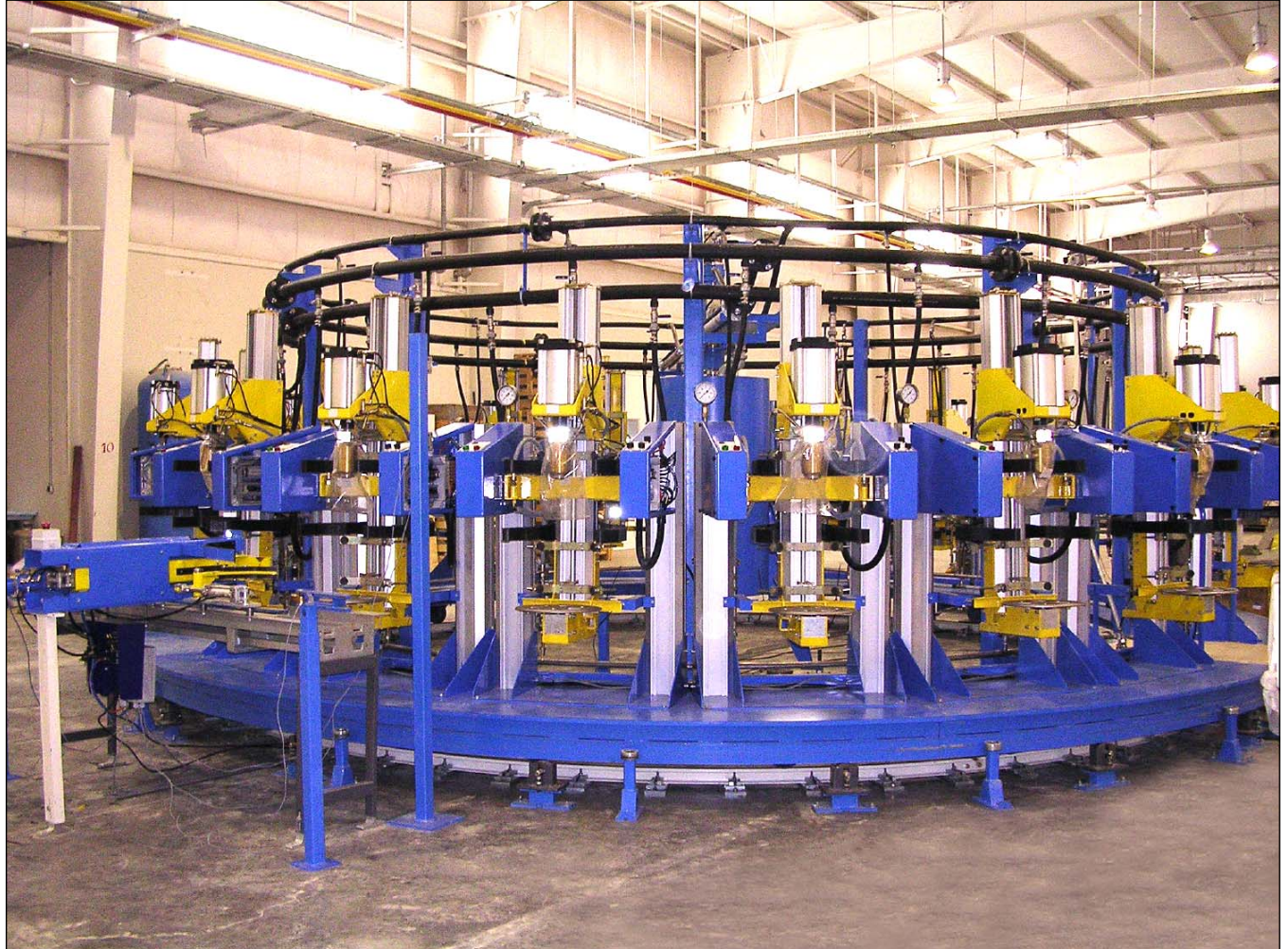
PTC pressure testing carousel for domestic cylinders
