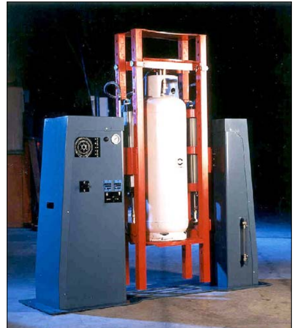
PTU pressure testing unit for industrial cylinders
