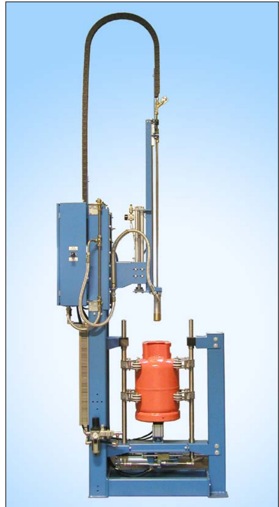
Combined machine for internal cleaning of LPG cylinders with steam and suction of residual water and dissolved dirt. The illustrated machine is to be installed in-line in chain conveyor and can handle two types of cylinders with different heights.
