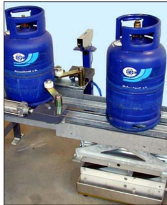
Detailed view of accumulation stop on chain conveyor (including photocell), underweight and lifting table
