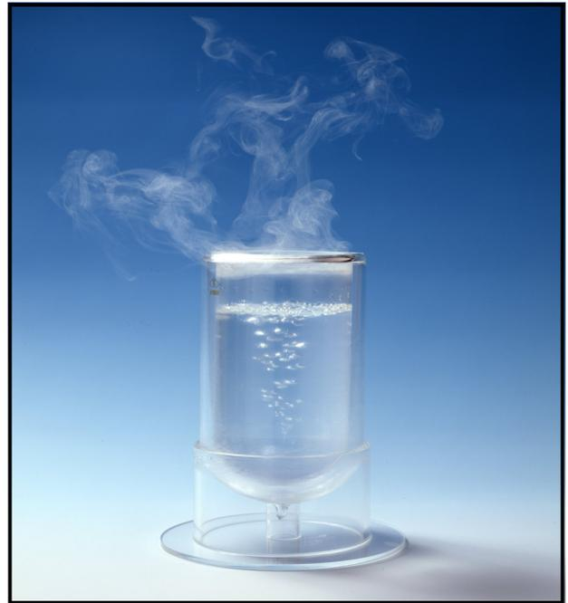
Figure 1. LNG “boiling” at atmospheric pressure and temperature (Source: Osaka Gas Co. Ltd.)
