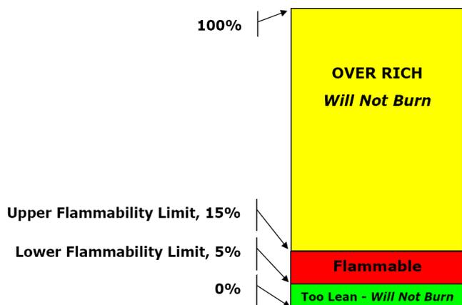
**Figure 4.** Flammability range for methane (Source: Foss 2003)
