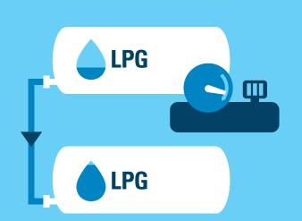
The compressor transfers the liquid between tanks by increasing the pressure in the first tank, causing the liquid gas to flow into a second tank.
