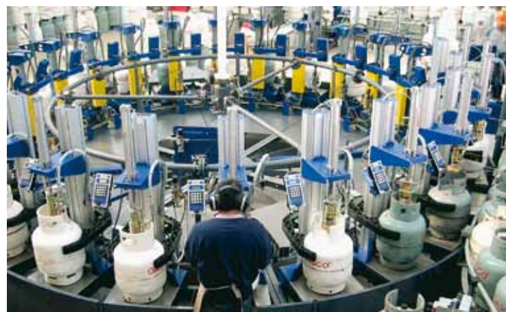
The UFM can be installed as a stationary unit on the floor, built into a chain or roller conveyor system or mounted on an existing or new carousel
