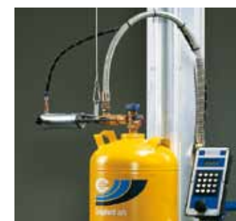
Optional installation of manual, semi-automatic or fully automatic filling heads
