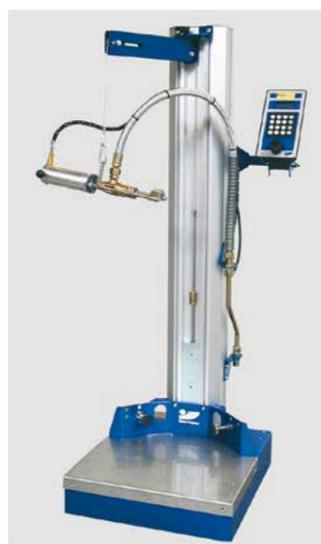
*UFM for manual filling of industrial cylinders with screw valves*
