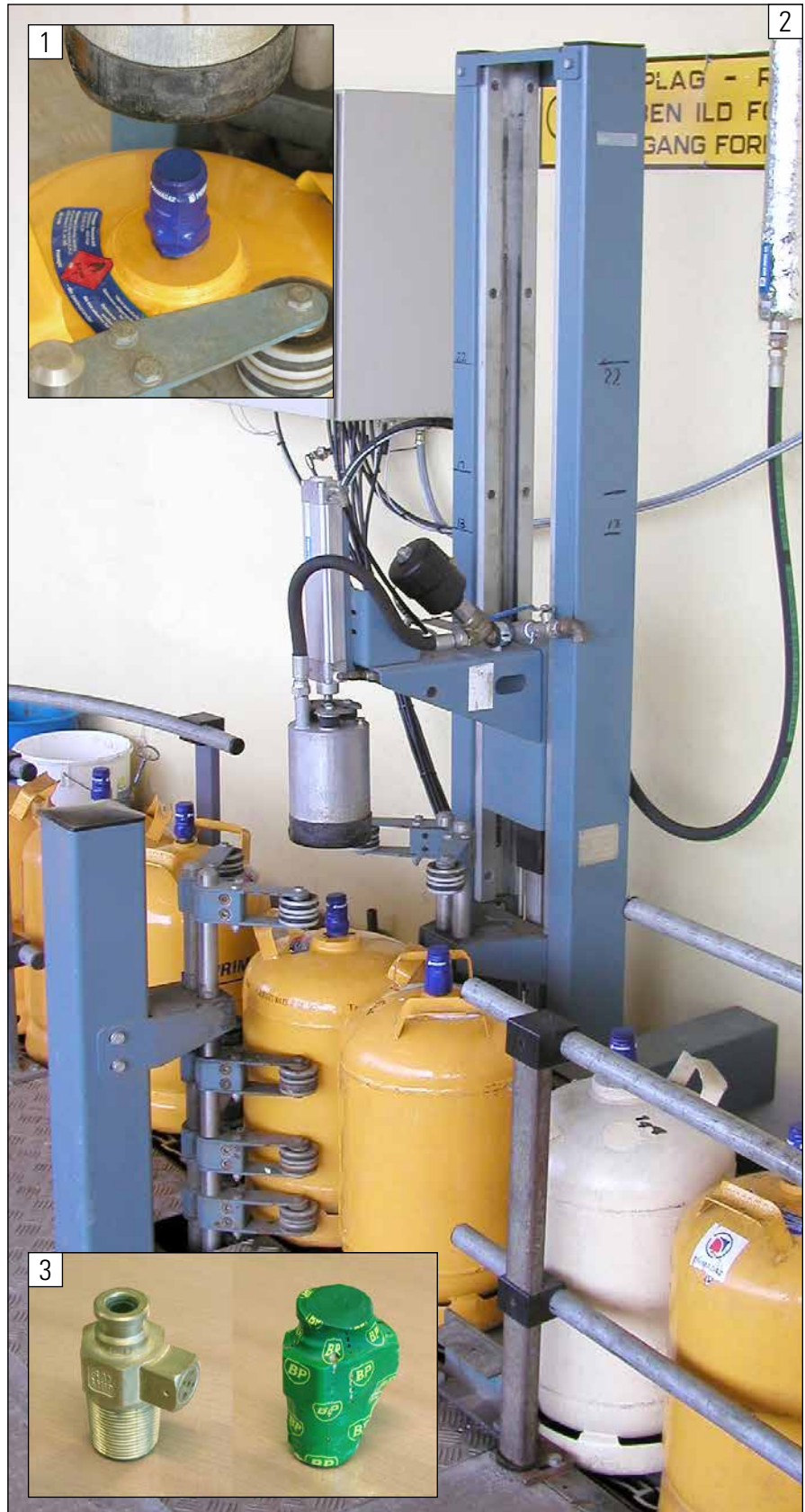
The fully automatic SMS thermosealing machine, which shrinks seals by means of water steam, is designed for installation in a chain conveyor
