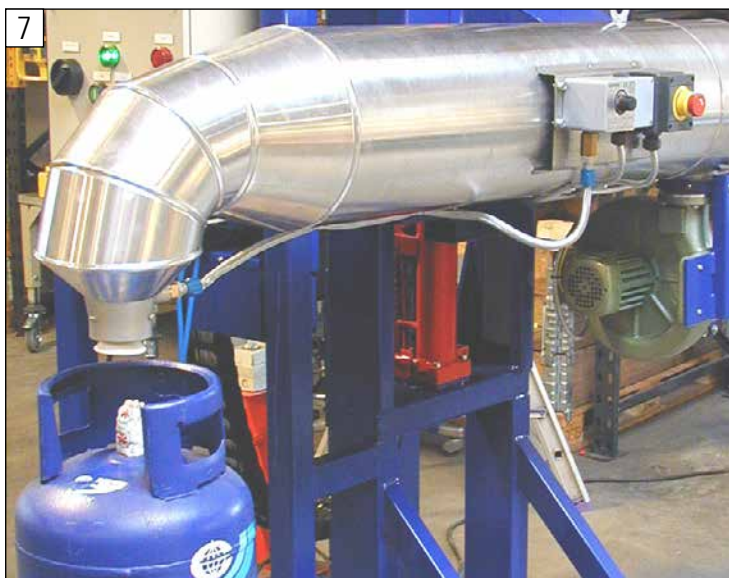
The fully automatic SMA thermosealing machine, which shrinks seals by means of hot air, is designed for installation in a chain conveyor
