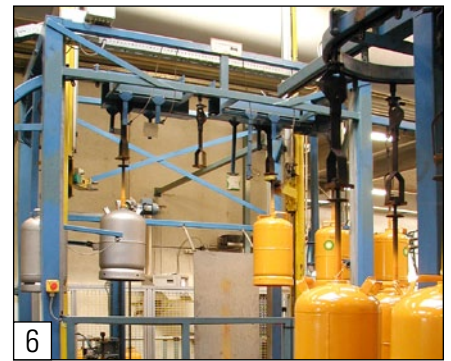
Automatic transfer of cylinders from chain conveyor system to overhead conveyor system
