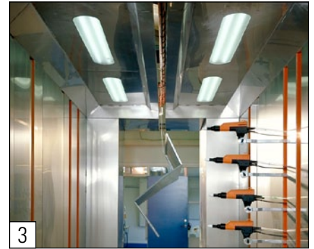
Spray booth for automatic application and recovery of powder paint
