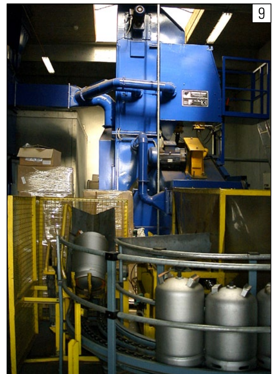
Shotblasting equipment with automatic loading and unloading of cylinders
