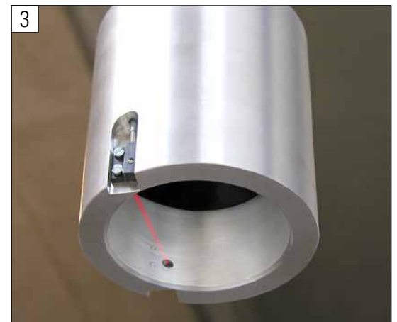
The orientation head is lowered upon the valve and the cylinder is rotated. When the valve is in the right position inside the orientation head, a fibre optic beam (on the picture shown as a read beam) is cut off, and the cylinder stops rotating.
