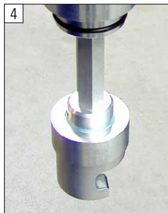
Each valve changing key can be fitted to the valve type in question (or possibly to the valve types in question)
