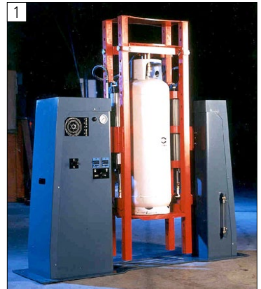
PTU pressure testing unit for industrial cylinders
