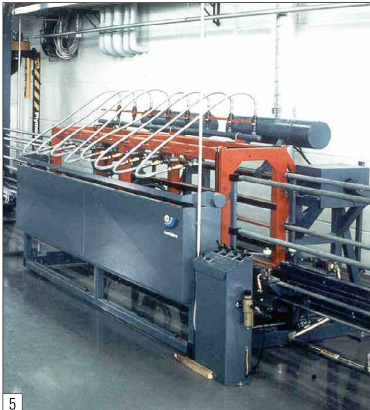
In-line ERI evacuation system integrated in chain conveyor
