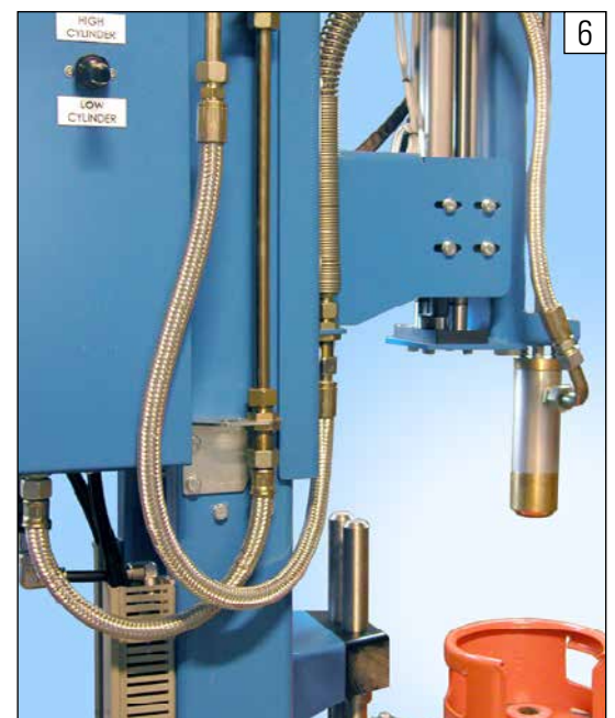
Combined machine for internal cleaning of LPG cylinders with steam and suction of residual water and dissolved dirt. The illustrated machine is to be installed in-line in chain conveyor and can handle two types of cylinders with different heights.
