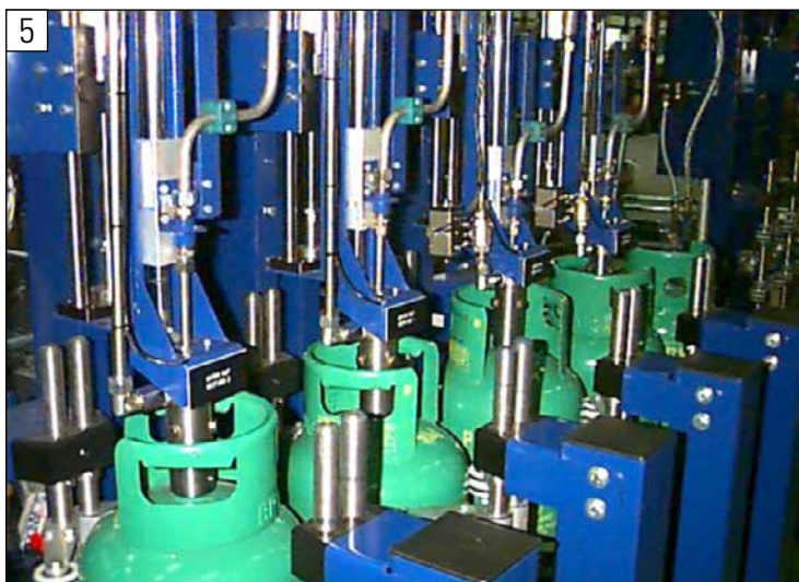
Equipment for internal cleaning of LPG cylinders installed in-line in chain conveyor
