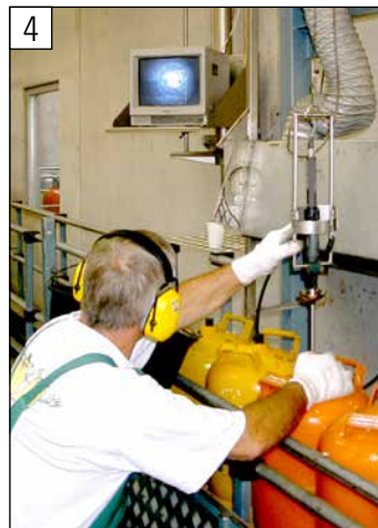
Equipment for internal inspection of LPG cylinders installed in-line in chain conveyor
