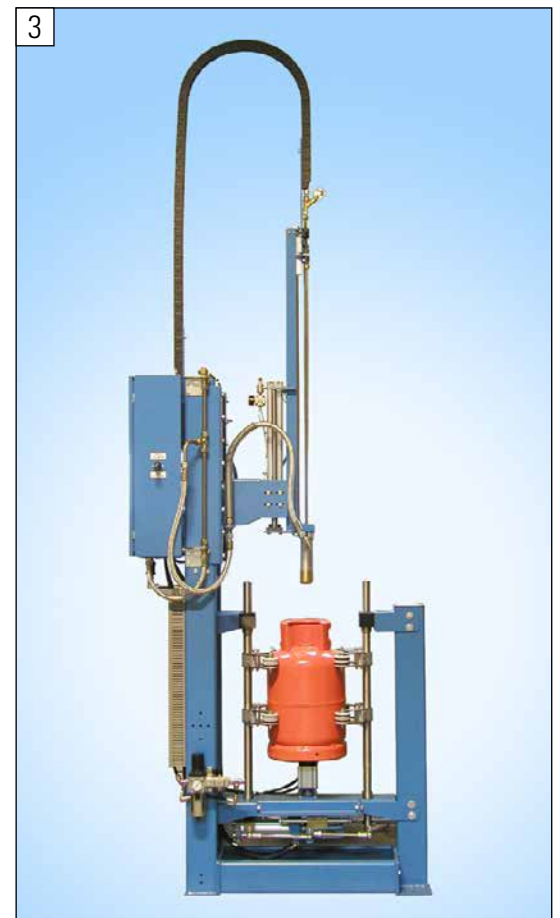
Combined machine for internal cleaning of LPG cylinders with steam and suction of residual water and dissolved dirt. The illustrated machine is to be installed in-line in chain conveyor and can handle two types of cylinders with different heights.
