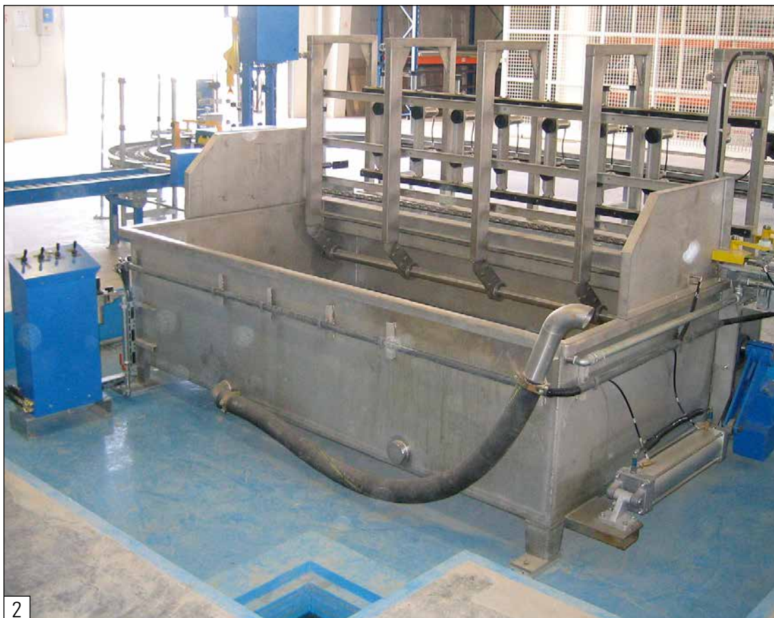
Semi-automatic pneumatic EB-8 leak testing bath integrated in chain conveyor with discharge of leaky cylinders
