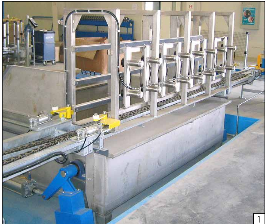
Semi-automatic pneumatic EB-8 leak testing bath integrated in chain conveyor with discharge of leaky cylinders
