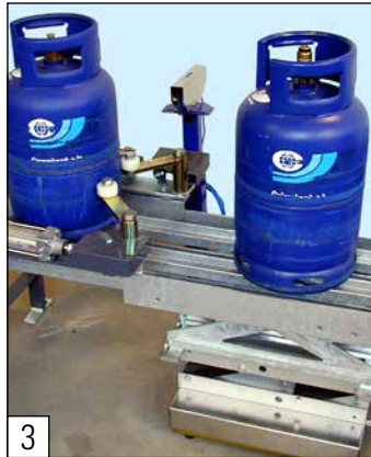
3 Detailed view of accumulation stop on chain conveyor (including photocell), underweight and lifting table
