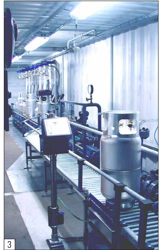
3 In-line filling system with roller conveyor
