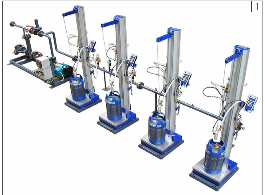
One-man LPG filling unit with four UFM universal filling machines and complete platform with LPG pump unit, ex-proof power panel and piping arrangement (incl. filter, differential pressure valve and LPG liquid level sensor)
