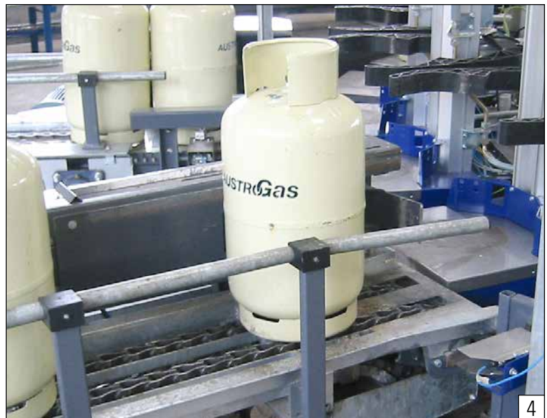
PER ejection unit for radial ejection of cylinders from filling carousel
