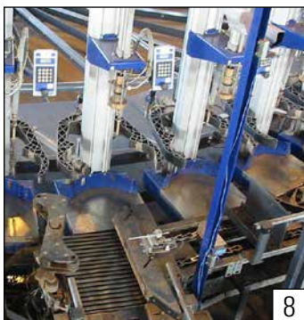
Radial introduction unit combined with tangential ejection unit with a cylinder pusher on each filling machine
