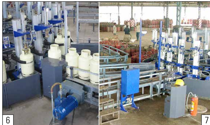
Carousel filling systems with radial introduction and ejection units
