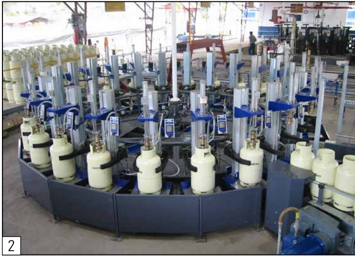
2 Carousel filling system with UFM universal filling machines
