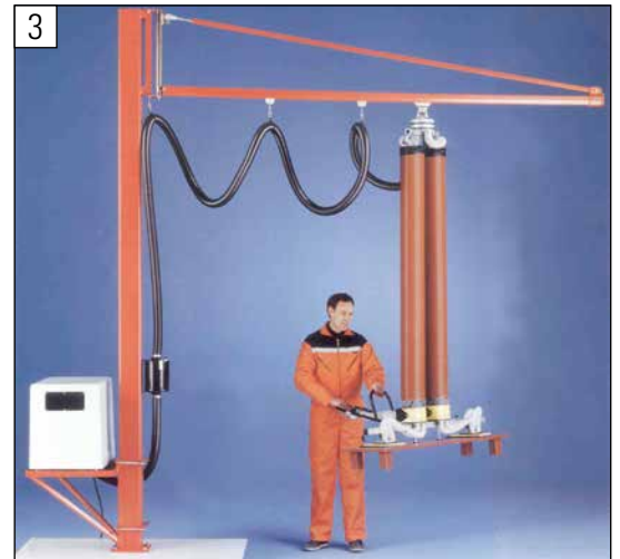
Example of suspension device for an overhead handling system based on the vacuum principle
