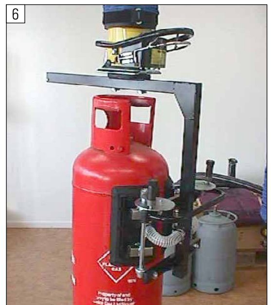
Handling system, based on the vacuum principle, for one cylinder
