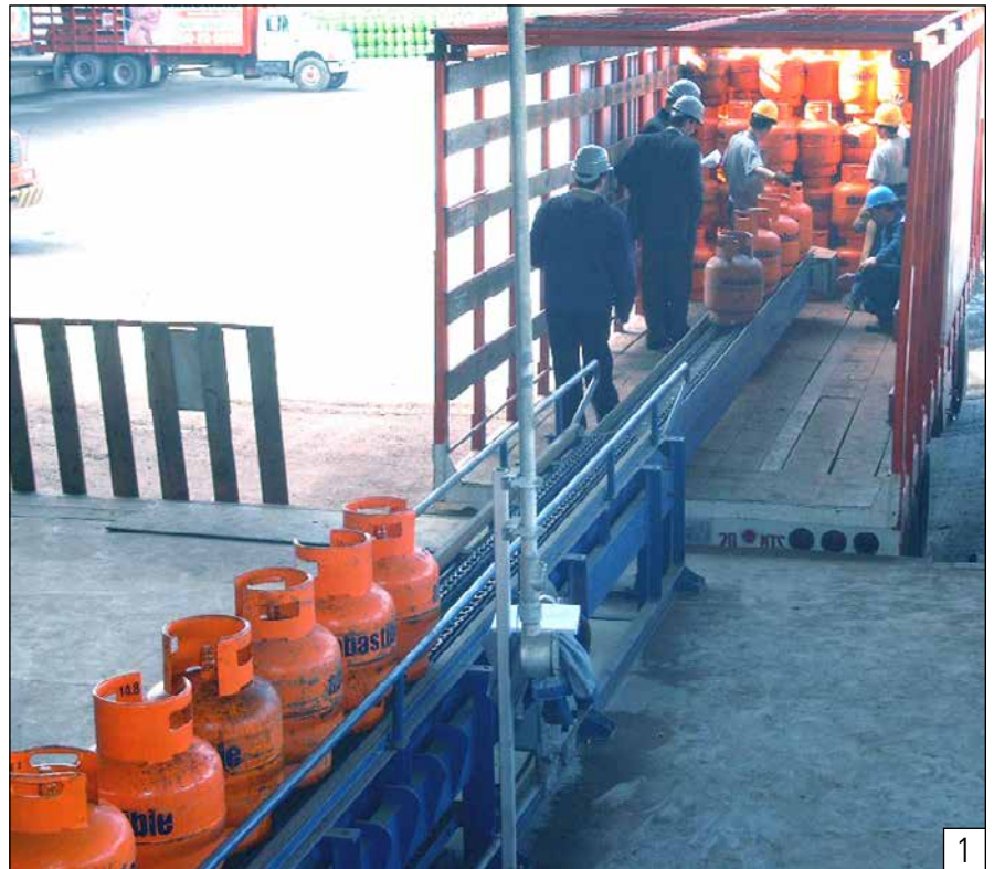
Kosan Crisplant's telescopic conveyor has been designed to facilitate the heavy manual handling in connection with loading/unloading of LPG cylinders onto/from trailers or lorries. The conveyor is mounted as a direct extension of the chain conveyor on the platform or the ramp. It consists of a stationary section as well as a movable section in the form of a built-in telescopic extension.
