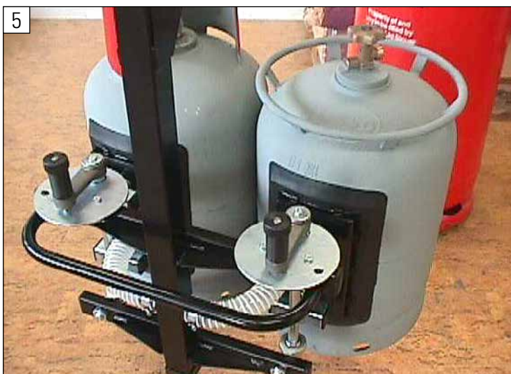
Handling system, based on the vacuum principle, for two cylinders
