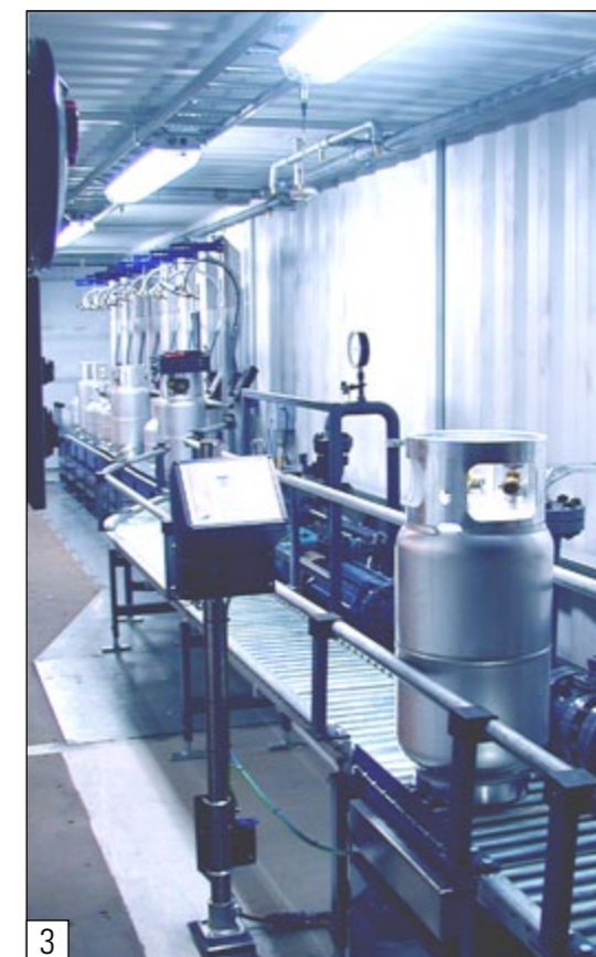
In-line filling system with roller conveyor
