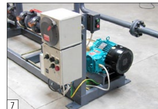
Ex-proof power panel for LPG pump unit
