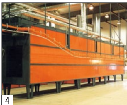
Tunnel oven for drying after pre-treatment, curing/drying wet paint or curing powder paint
