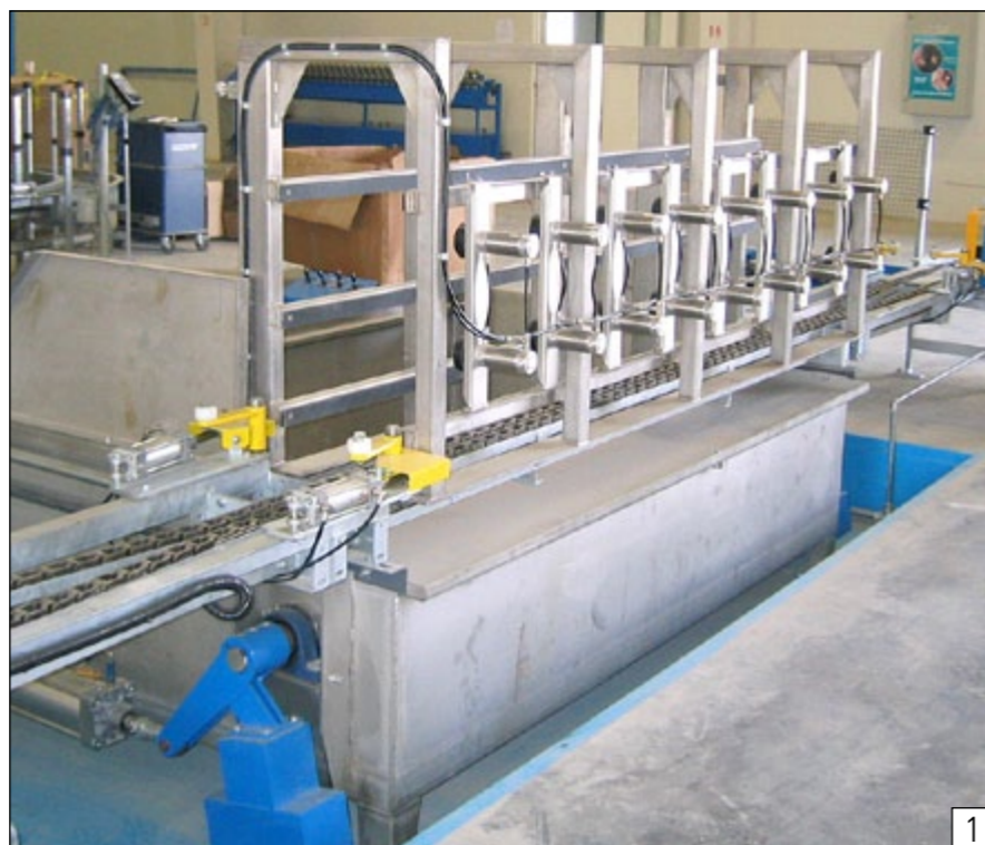
Semi-automatic pneumatic EB-8 leak testing bath integrated in chain conveyor with discharge of leaky cylinders
