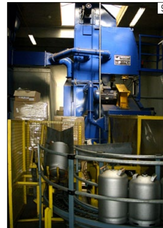
Shotblasting equipment with automatic loading and unloading of cylinders
