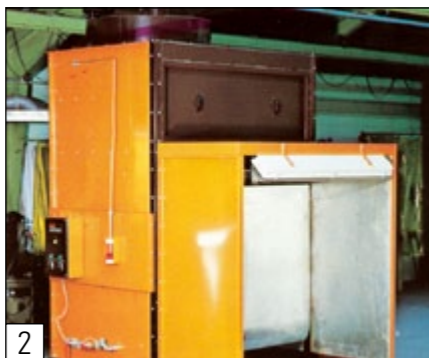
Spray booth for manual application of wet paint
