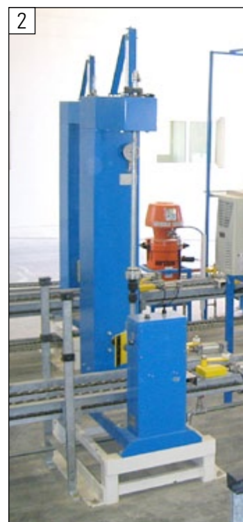
PVS valve changing machine for installation in chain conveyor
