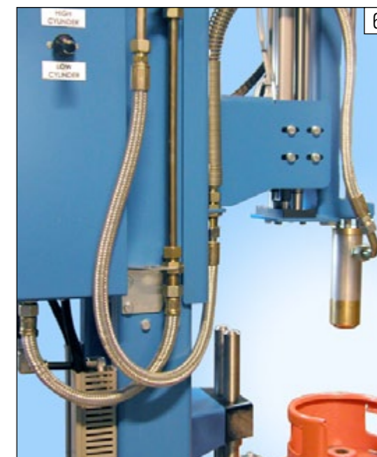
Combined machine for internal cleaning of LPG cylinders with steam and suction of residual water and dissolved dirt. The illustrated machine is to be installed in-line in chain conveyor and can handle two types of cylinders with different heights.
