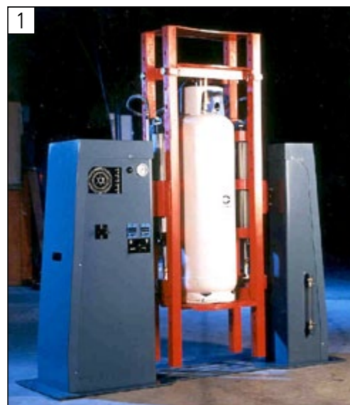
PTU pressure testing unit for industrial cylinders
