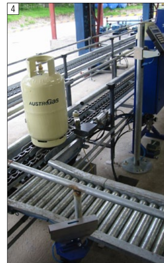
Fully automatic ECS check weighing system installed in-line in chain conveyor with roller conveyor for ejection of incorrectly filled cylinders
