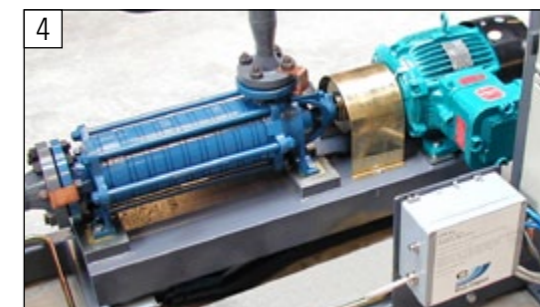
LPG pump unit, ex-proof electrical motor and Kosan Crisplant's CPI power supply for intrinsically safe network
