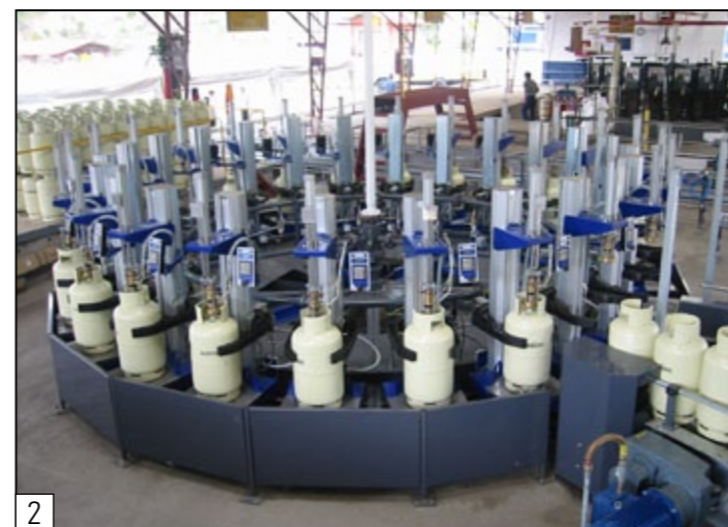
Carousel filling system with UFM universal filling machines
