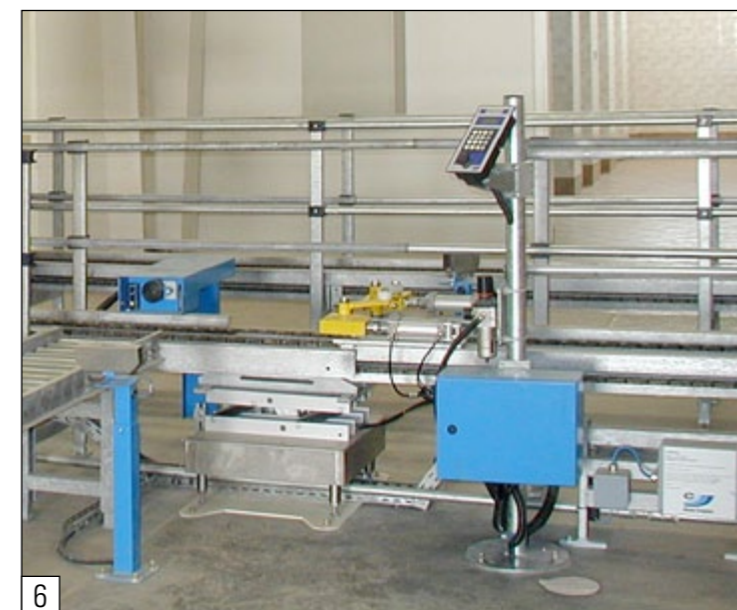
Fully automatic ECS check weighing system installed in-line in chain conveyor with automatic ejection of incorrectly filled cylinders
