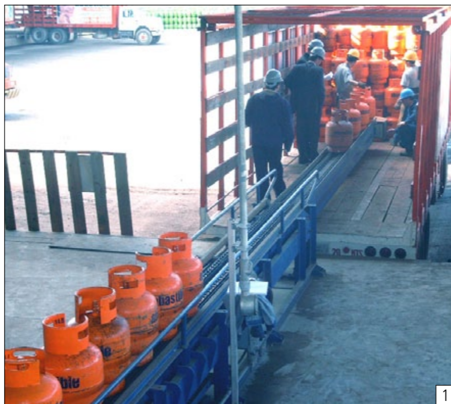
Kosan Crisplant's telescopic conveyor has been designed to facilitate the heavy manual handling in connection with loading/unloading of LPG cylinders onto/from trailers or lorries. The conveyor is mounted as a direct extension of the chain conveyor on the platform or the ramp. It consists of a stationary section as well as a movable section in the form of a built-in telescopic extension.
